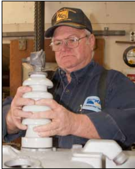
Danny Seele, KEC's director of Apparatus Testing, puts in a bushing in a three-phase recloser.
